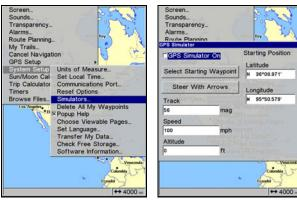
Simulators highlighted on System Setup menu (left). GPS Simulator on selected on Simulators menu (right).
